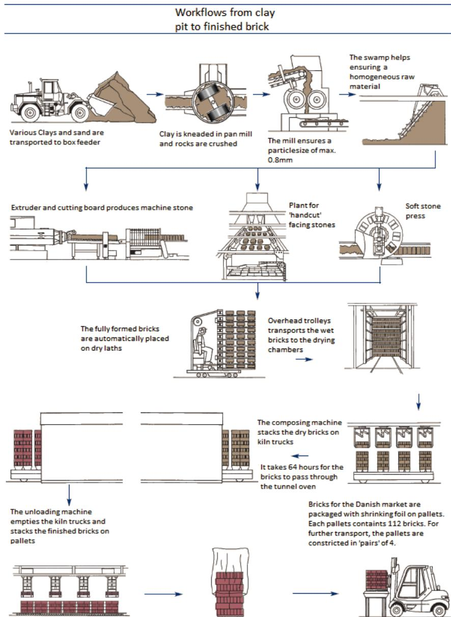
The flow diagram conforms with the requirements in the modular approach and shows the production phase A3 for brick production (Petersminde Teglværk only uses "soft stone press", no "extruder" and no "handcut"). The remaining phases are described below.
